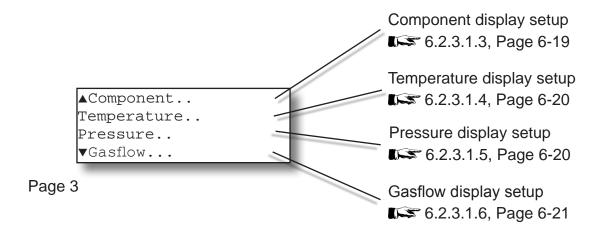
Beginning with rev. 1.1, X-STREAM X2 supports 2 measurement display pages, to show additional measuring results. To configure this 2<sup>nd</sup> page, enter menu page 4 of the current menu.
